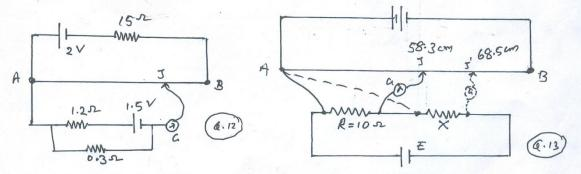
Q.13 Fig shows a potentiometer circuit for comparison of two resistances. The balance point with a standard resistor  $R=10\Omega$  is found to be 58.3 cm, while that with the unknown resistance X is 65.5cm.
