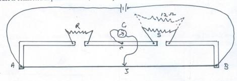
Q.8) In a meter bridge experiment, resistors of resistance  $5\Omega$  and  $2\Omega$  are connected in the left and right gap respectively. When the resistor of  $5\Omega$  is shunted by a wire, the balance point is found at 62.5cm mark. What is the resistance of the wire?
